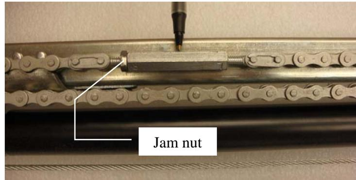
Warning: Thread lock was applied at the factory which could make the nut and turnbuckle difficult to turn. Take care not to break the bolt, ensure the bolt is not twisting and is threading as it will shear off. It will help dramatically if a penetrating oil is sprayed on this area.
