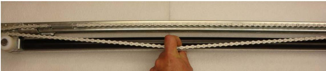
4. After all four jacks have been adjusted run the unit up and down a couple times, this might require some additional weight applied to the top of the jack in the down stroke to help compress the gas cylinders.
