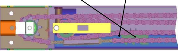
Position the shim back between the chain holder and the interior tube.
