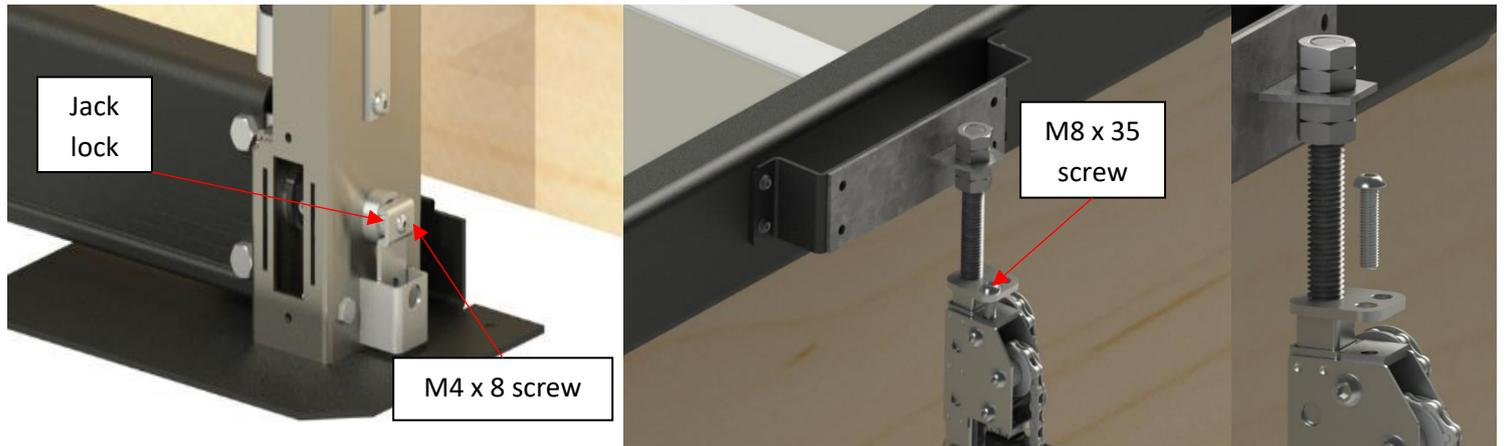
12) Once the U-frame is in place, you can now remove the jack lock bracket at the bottom of the non-motor jack. Unscrew the Philips M4 x 8 mm bolt. **Keep the lock bracket and the hardware for future use.** If your unit doesn't have a jack lock bracket near the bottom of the jack (model 2019 and +), locate the M8 x 35mm screw at the top and remove it to unlock the jack assembly.
