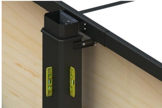
20) Attach the top cover of the two posts. Use the provided Robertson #8 self-drilling screws. (2 screws per post)
