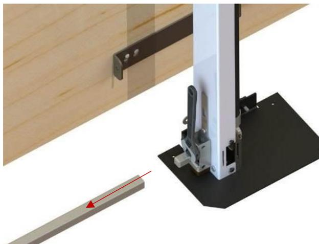
11) Fix an adjustable wrench to the square shaft of the non-motor jack.
