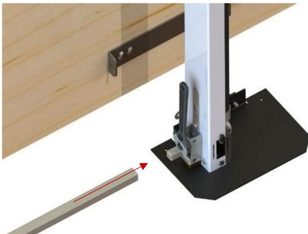
10) Install the U-frame over the drive shaft. The U-frame will bolt on the motor and on the non-motor jack. Fasten it back in place using the four hexagonal 5/16 in-18 x 2 in bolts and the 5/16 in-18 nylon insert locknuts. Use a 1/2 in socket wrench and spanner again.
