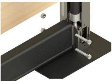
10) Take the drive shaft off. Slightly tilt the post to facilitate the operation.
